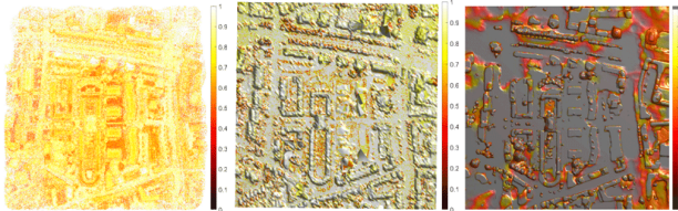
(b) Semantic uncertainty. Color shows the most likely class probability; higher values imply more certainty. L-R: PC, mesh, voxels. Figure 3: Enschede scene models and semantic uncertainty.
