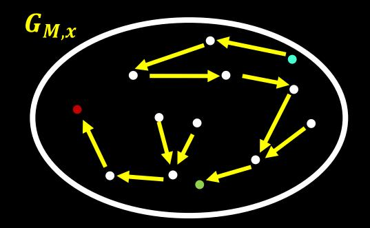
M accepts  $x \Leftrightarrow$  there is a path in  $G_{M,x}$  from the initial configuration node to a node in an accept state
