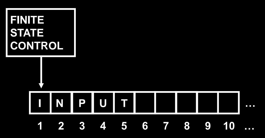
We measure *space* complexity by finding the *largest tape index reached* during the computation
