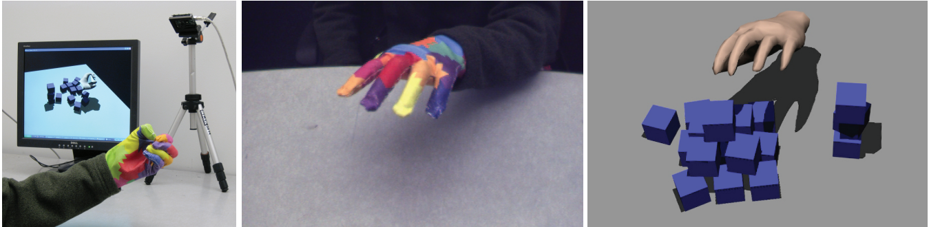
Figure 1: We describe a system that can reconstruct the pose of the hand from a single image of the hand wearing a multi-colored glove. We demonstrate our system as a user-input device for desktop virtual reality applications.
