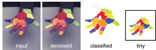
Figure 6: We denoise the input image before using a mixture-of-Gaussians color classifier to segment the hand. Our normalization step consists of cropping and rescaling the hand region into a 40 \times 40 tiny image.
