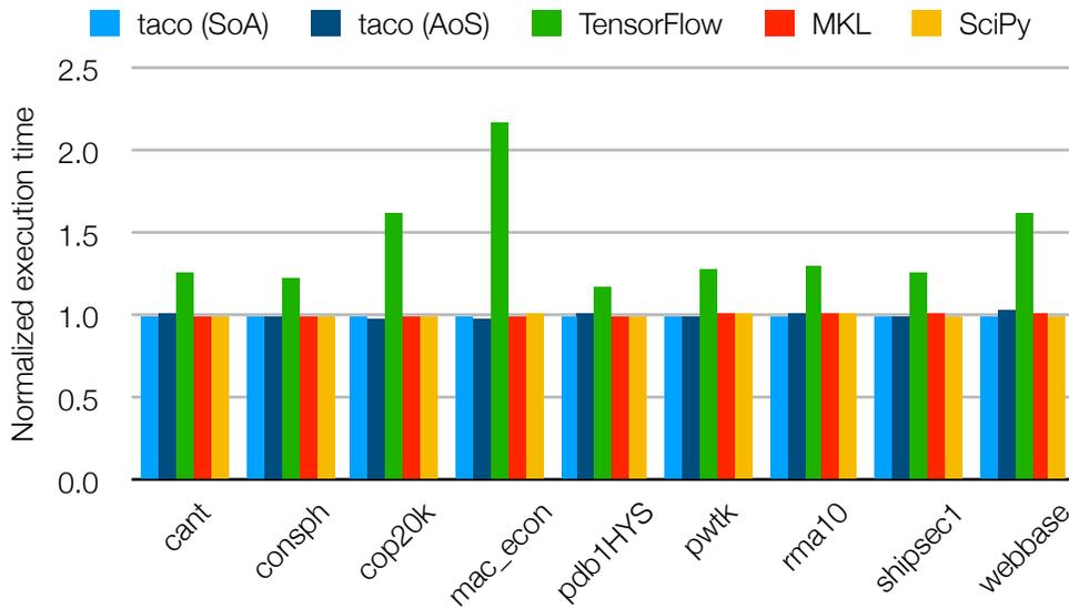
Figure 5-1: Normalized execution time of COO SpMV ( $y = Ax$ , where  $A$  is a COO matrix and  $x$  and  $y$  are dense vectors) with our technique (taco) and existing sparse linear algebra libraries, relative to taco with SoA COO for each matrix.
