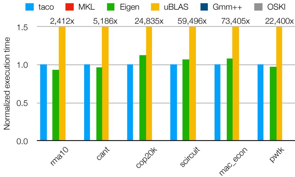
Figure 5-6: Normalized execution time of CSR SDDMM ( $A = B \circ (CD)$ , where  $A$  and  $B$  are CSR matrices and  $C$  and  $D$  are dense matrices) with our technique (taco) and existing sparse linear algebra libraries, relative to taco for each matrix. We omit results for libraries that do not support the computation.
