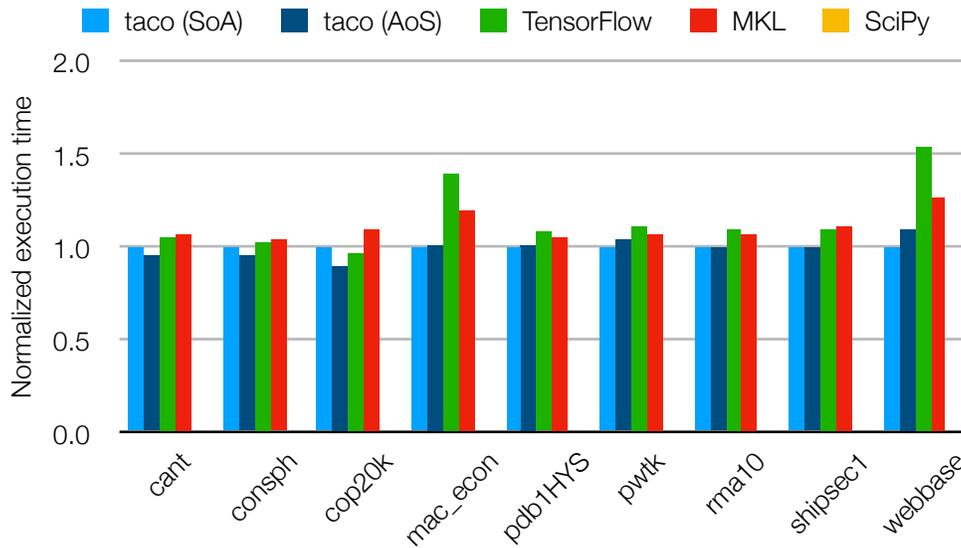
Figure 5-2: Normalized execution time of COO SpDM ( $A = BC$ , where  $B$  is a COO matrix and  $A$  and  $C$  are dense matrices) with our technique (taco) and existing sparse linear algebra libraries, relative to taco with SoA COO for each matrix. We omit results for SciPy as it does not support computing SpDM directly on COO matrices.
