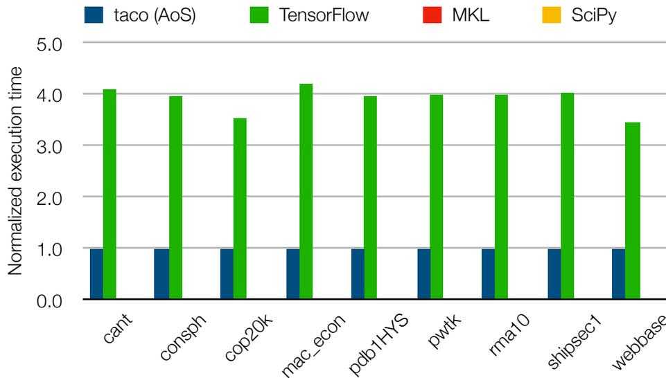
Figure 5-3: Normalized execution time of COO matrix addition ( $A = B + C$ , where the inputs and output are all stored in the AoS variant of the COO format) with our technique (taco) and TensorFlow, relative to taco for each matrix. We omit results for Intel MKL and SciPy as neither supports computing matrix addition directly on COO matrices.
