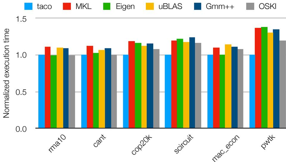
Figure 5-7: Normalized execution time of CSR RESIDUAL ( $y = b - Ax$ , where  $A$  is a CSR matrix and  $b$ ,  $x$ , and  $y$  are dense vectors) with our technique (taco) and existing sparse linear algebra libraries, relative to taco for each matrix.
