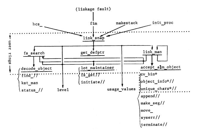
Underlined procedures are part of the proposed bound linker and will execute in the ring where a link is to be snapped.
