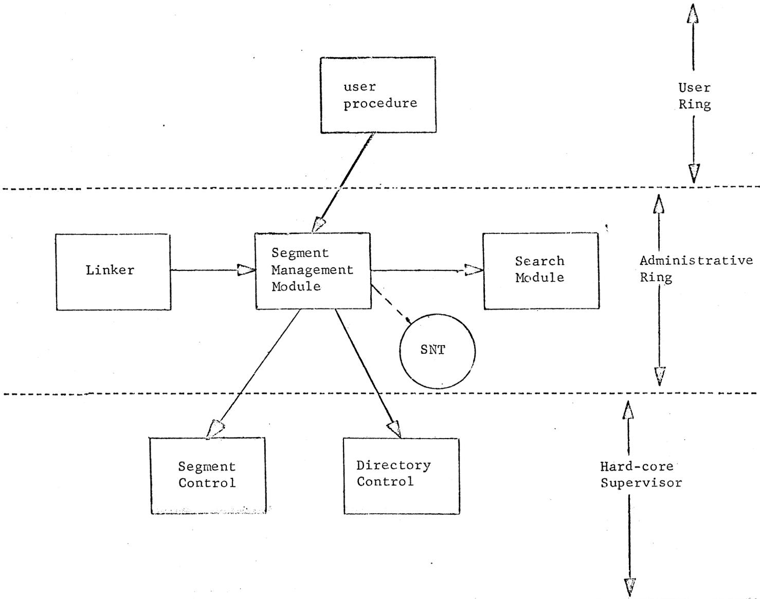
Figure I - The Segment Management Module's Interfaces
