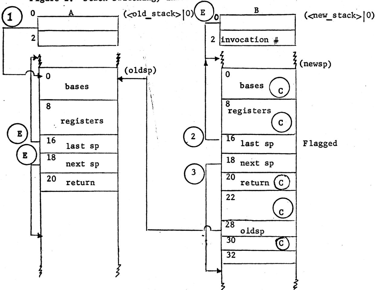
Stack A belongs to the ring of the calling-procedure (old\_ring), stack B to the target procedure (new\_ring).
