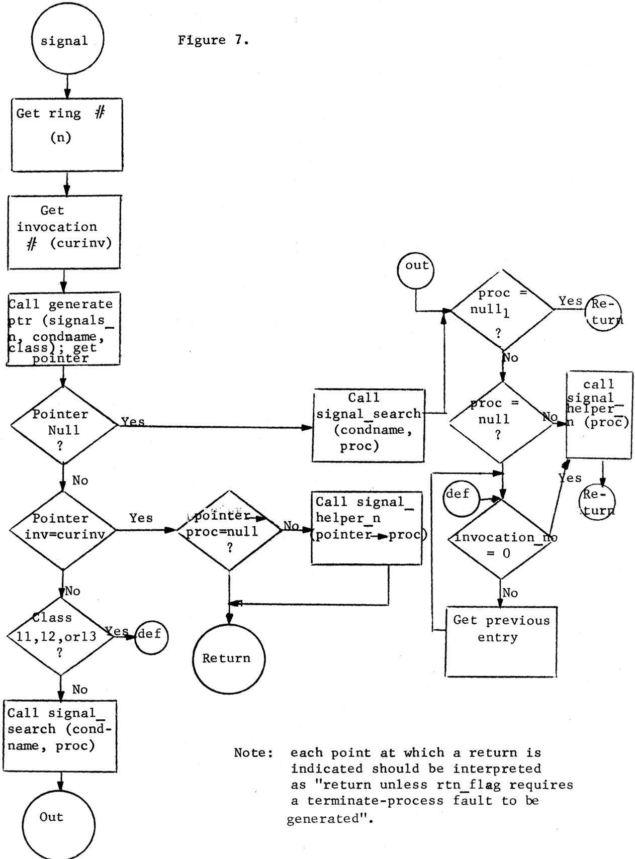
Note: each point at which a return is indicated should be interpreted as "return unless rtn\_flag requires a terminate-process fault to be generated".
