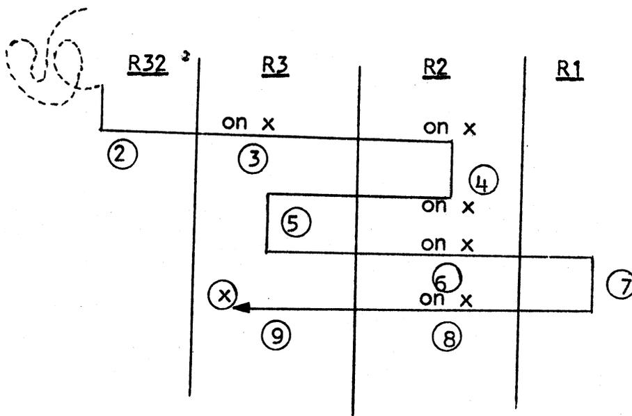
The wandering arrow represents control in a process, circled numbers are invocation numbers, "on x" indicates a call to condition for a condition named x. (The  $R_i$  are protection rings.)
