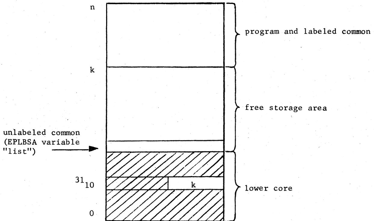
Figure 1: Loading diagram for EPLBSA.
