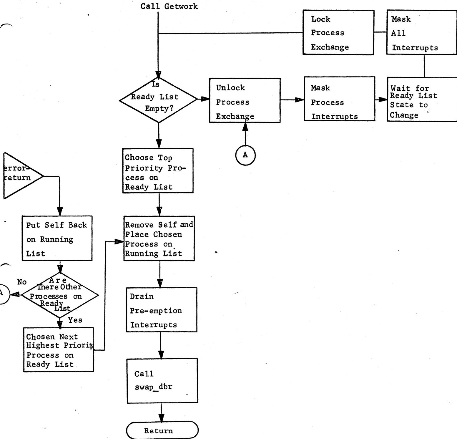
Figure 2. Basic Outline of Getwork with Additions to Enable Unloading of Processes
