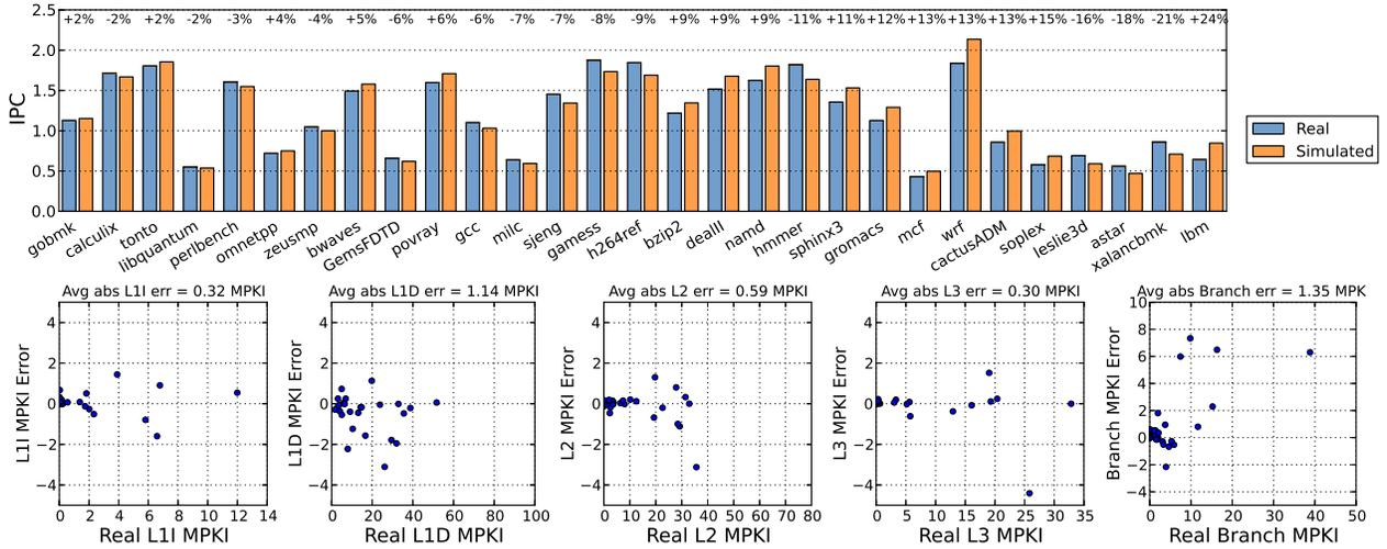
Figure 5: Validation of the OOO core model against a real Westmere machine on SPEC CPU2006: Simulated vs real IPC, and scatter plots of per-application MPKI errors (simulated - real MPKI) for all the caches and the branch predictor.
