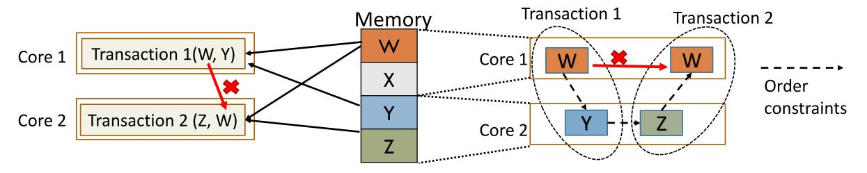
Shared memory system → coherence protocol Coherence poorly suited for accelerators
