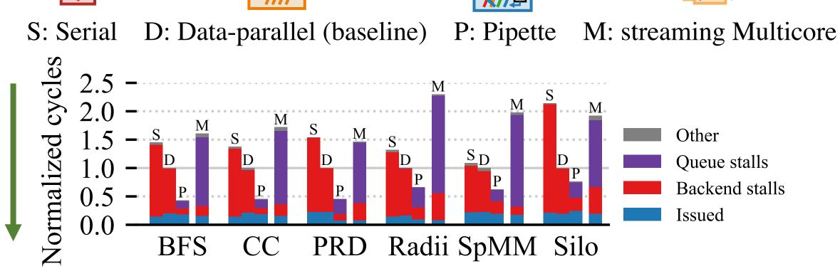
Pipette reduces impact of memory latency (**smaller red bars**) and load imbalance (**smaller purple bars**)
