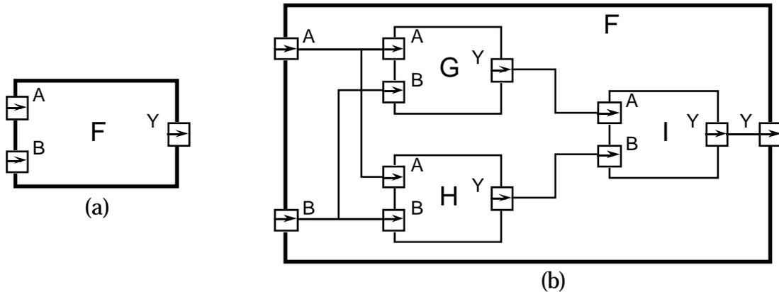
Figure 1-1. Example of a structural description.
