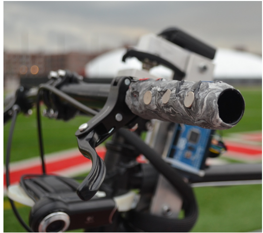
FIG. 6. Vibrating handlebars. Note the metallic vibration motors attached via sugru to the forward side of the handlebars. Wiring is routed internally for aesthetics and safety.
