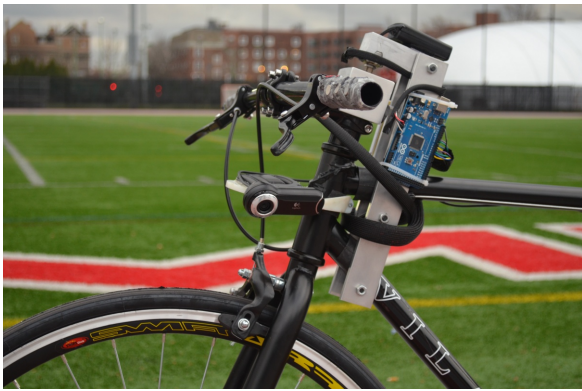
FIG. 2. Main components of bicycle. The camera is used to localize the bike with respect to the track edge. Custom vibrating handlebars are controlled by a microcontroller and drive circuitry. The steering angle of the bicycle is also measured by a microcontroller and relayed to an onboard laptop in the rider’s backback. This laptop processes all sensor data, generates a target desired steering angle for bicycle, and sends commands to the handlebar motors via the microcontroller.
