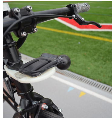
FIG. 8. The sideways-facing camera monitors the track/pavement border.
