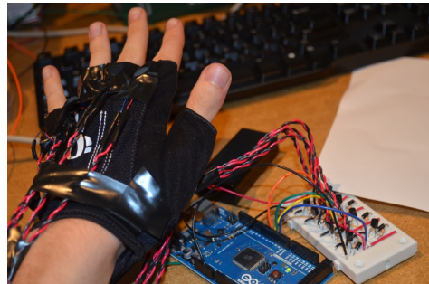
FIG. 4. Vibrating glove prototype. Each finger has a vibration motor and is individually controllable with PWM.
