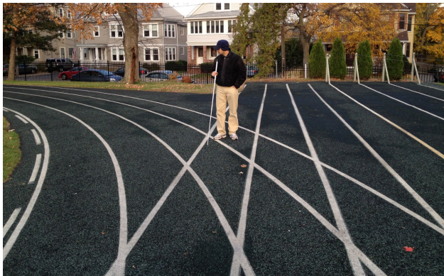
FIG. 7. A curved, hashing pattern produced by normal lanes and merging starter lanes at the Perkins track. These pose a significant challenge for lane-tracking algorithms. Unfortunately, these problematic areas occur at the areas of highest rider danger along the track and hence motivated our decision to use the inner grass / pavement border for computer vision instead of the white lanes.
