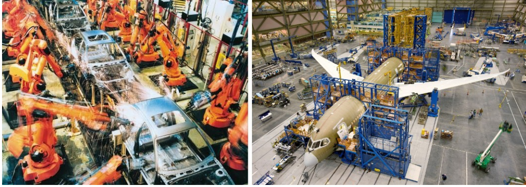
Figure 3-1: At left, an illustration of a mass-production automotive facility. The robots execute the same task repeatedly with no variation, thanks to a precisely-designed environment where nearly all variability is engineered away. At right shows a typical modern aircraft manufacturing facility. Due to the different nature of the product being produced, mass-manufacturing techniques and a highly-engineered environment aren't easily implementable.
