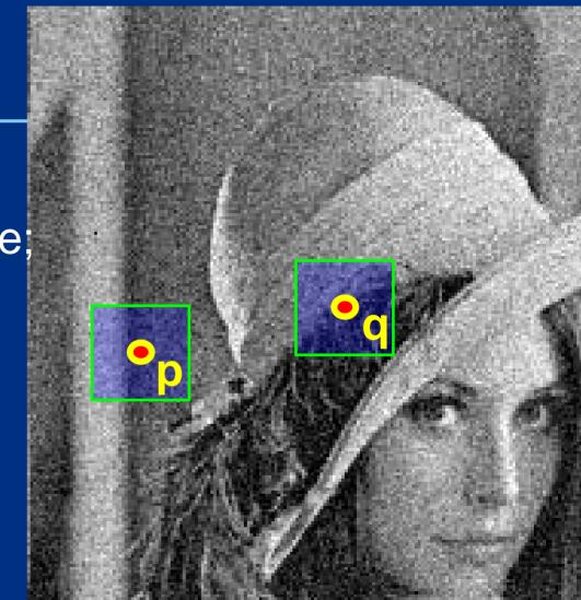
$$NLMF [I]_{\mathbf{p}} = \frac{1}{W_{\mathbf{p}}} \sum_{\mathbf{q} \in S} G_{\sigma_{\mathbf{r}}} \left( \| V_{\mathbf{p}}^{\boldsymbol{\rho}} - V_{\mathbf{q}}^{\boldsymbol{\rho}} \|^{2} \right) I_{\mathbf{q}}$$
