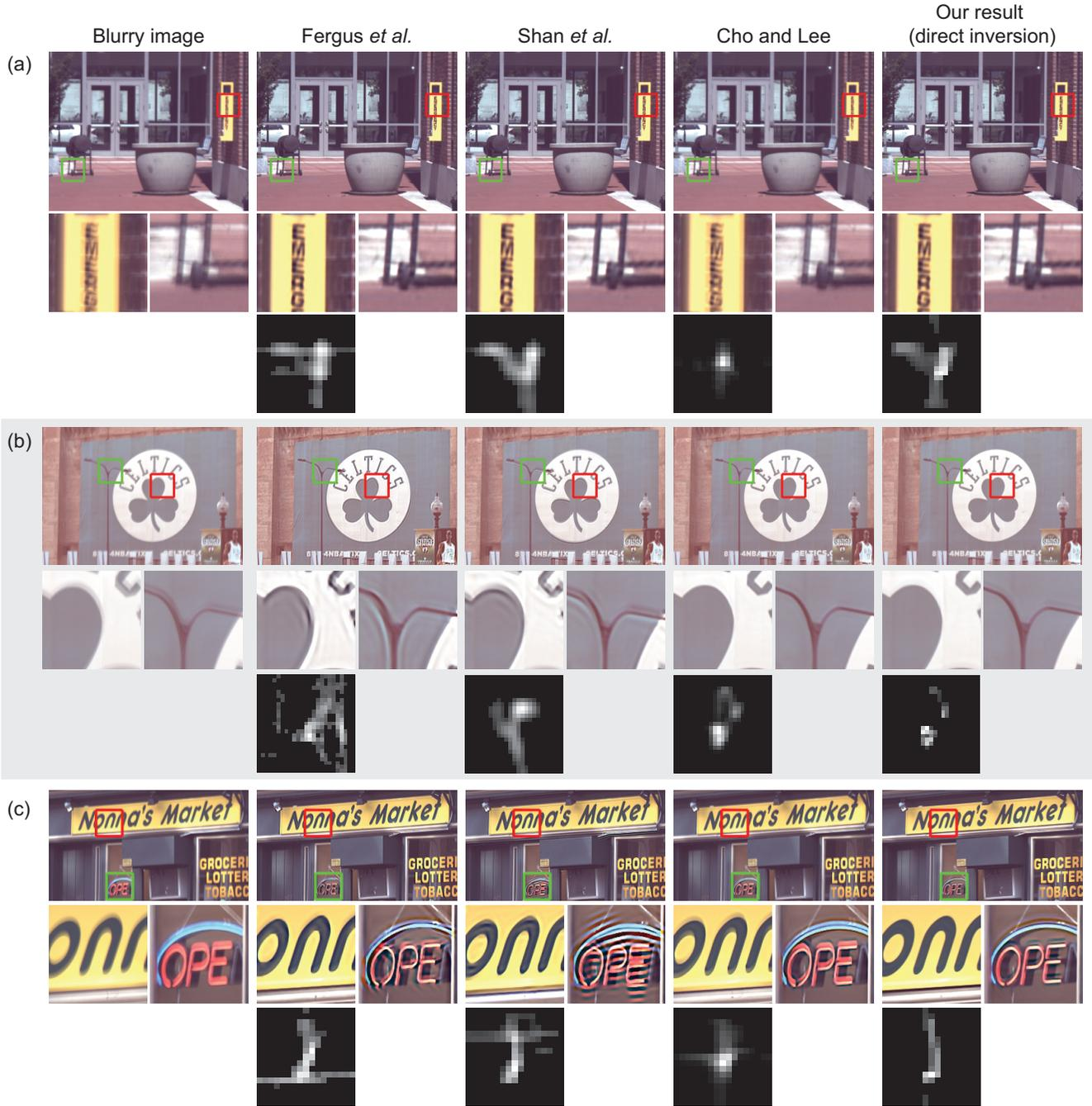
**Figure 5:** We compare our algorithm to the methods of Fergus et al. [4], Shan et al. [12], and Cho and Lee [2]. On this man-made environments, our algorithm compares favorably to prior art. These results may be better seen on the electronic version.
