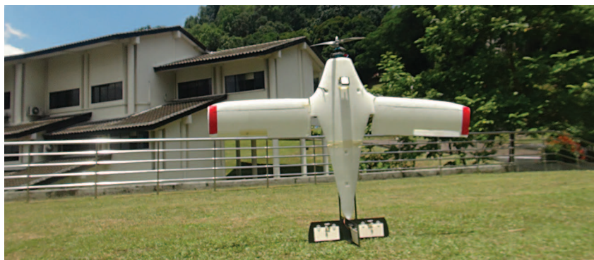
FIGURE 3. The U-Lion is a hybrid UAV that can take off and land vertically and fly horizontally at high speed.
