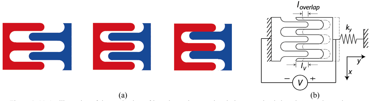
Figure 4. (a) An illustration of the mechanism of lateral snap-in occurring during operation below the normal snap-in voltages: (i) Normal position of the fingers of the combdrive at a given voltage (ii) Additional overlap created by a mechanical disturbance (iii) Snap-in at a voltage lower than the normal snap-in voltage, due to the presence of extra comb finger overlap that forces the structure into a laterally unstable domain. (b) Schematic of the combdrive showing the parameters used in the model.
