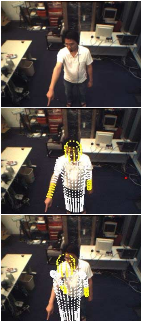
Figure 6: Original image (top) and tracking results from the audio-visual tracker (middle) and the standard vision-based (bottom) algorithms corresponding to frame 1860 of the sequence plotted in Figure 5. Around this frame, the user pronounced the word 'move', which induced a pointing context (right arm pointing, torso facing the projection screen).
