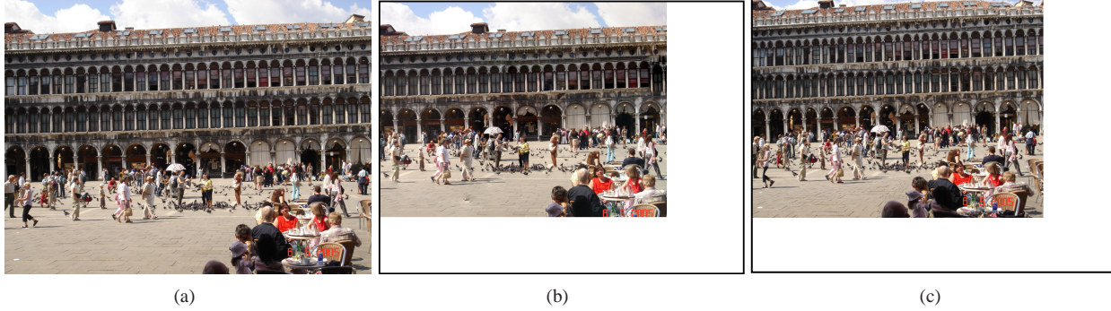
Figure 8. In this example, the original image shown in (a) is resized such that the width and height of the output image is 80% of the original image. (b) The reconstructed image from the patch transform framework. (c) The retargeting result using Seam Carving [2]. While Seam Carving preserves locally salient structures well, our work preserves the global context of the image through local evidence.
