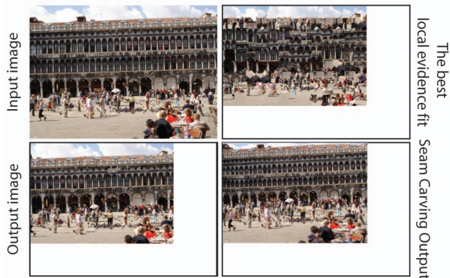
Fig. 6. The image retargeting example. The inverse patch transform reconstructs a resized image by solving for the patch assignment on a smaller canvas.
