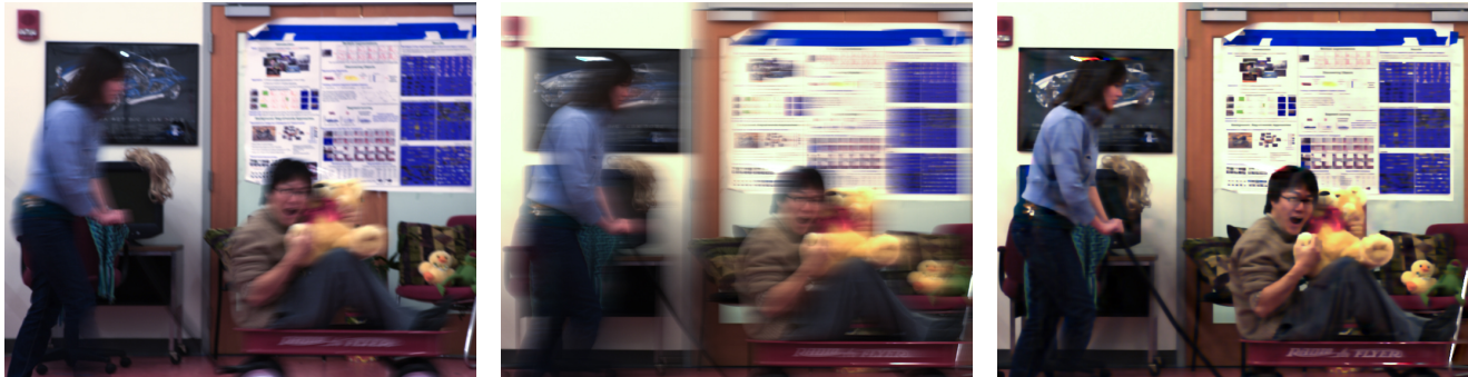
Figure 1: Left: Blurred motion captured by a static camera. Center: The same scene captured by a camera with a specially designed motion that causes both the static and dynamic regions to blur identically. Right: The blur from the center image can be removed independently of motion via deconvolution of the entire image with a single known point spread function.
