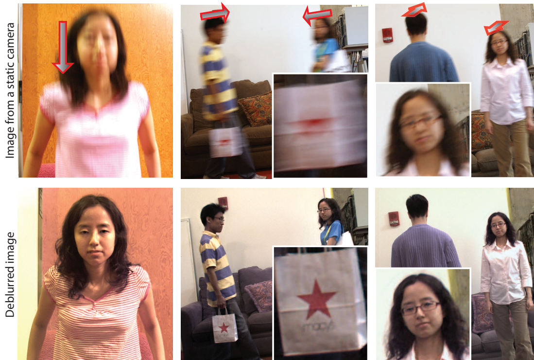
Figure 5.12: We show the deblurring performance of the orthogonal parabolic camera. Images from a static camera with 500ms exposure are shown for reference. Arrows on reference images show the direction and magnitude of motion.
