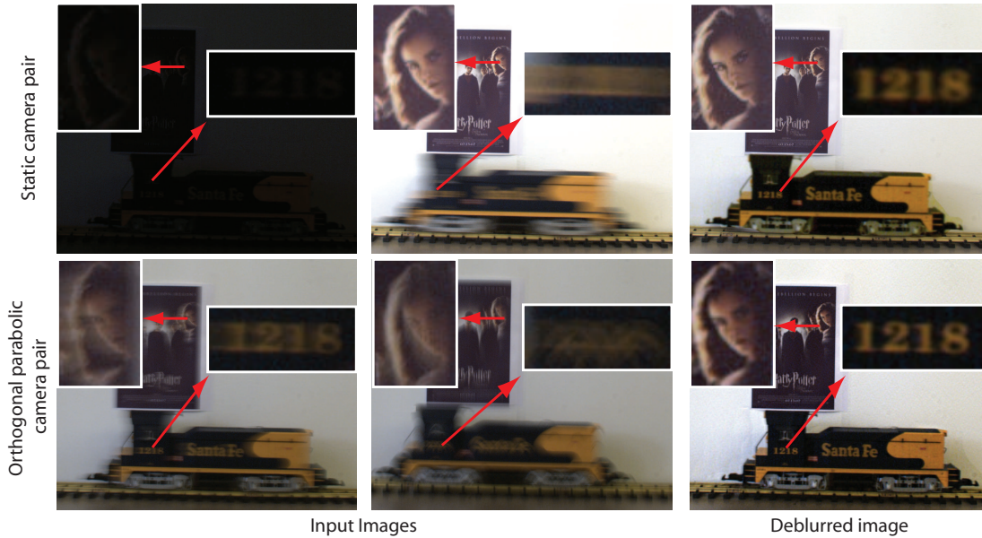
Figure 5.11: We compare the deblurring performance of a two-shot static camera and an orthogonal parabolic camera. We optimize the split of the exposure for the static camera, assuming that we know the object motion: 40ms for the first shot and 360ms for the second shot. The blur kernel is estimated manually to compare just the amount of information captured by these cameras. The static camera reconstructs static objects well, but at the expense of a degraded rendition of the moving object, whereas the orthogonal parabolic camera restores a reasonable rendition of both the static and moving parts.
