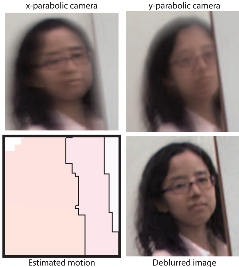
Figure 5.13: Our image reconstruction algorithm handles occlusion boundaries in a manner similar to motion boundaries. In the occluded region, an image deblurred using only one of the two input images is used.
