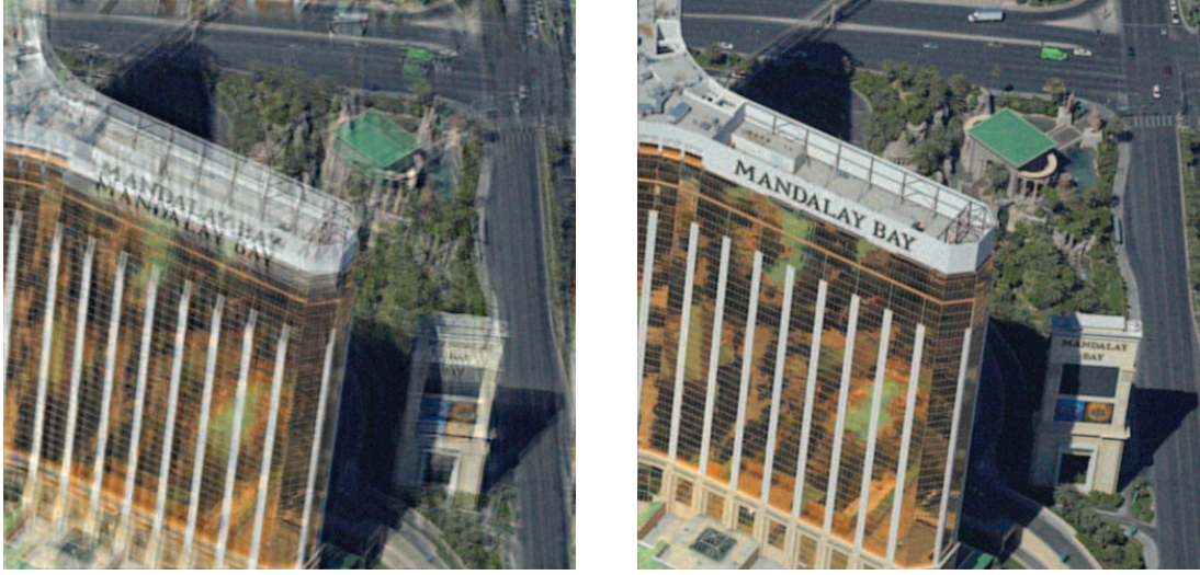
Figure 5.9: An image is synthetically blurred, and is deconvolved using the correct blur kernel pair and an incorrect blur kernel pair. An incorrect blur kernel pair has a spatial shift incompatible with input images, leading to ghosting and ringing in the restored image, whereas the correct kernel pair restores a sharp, artifact free image.
