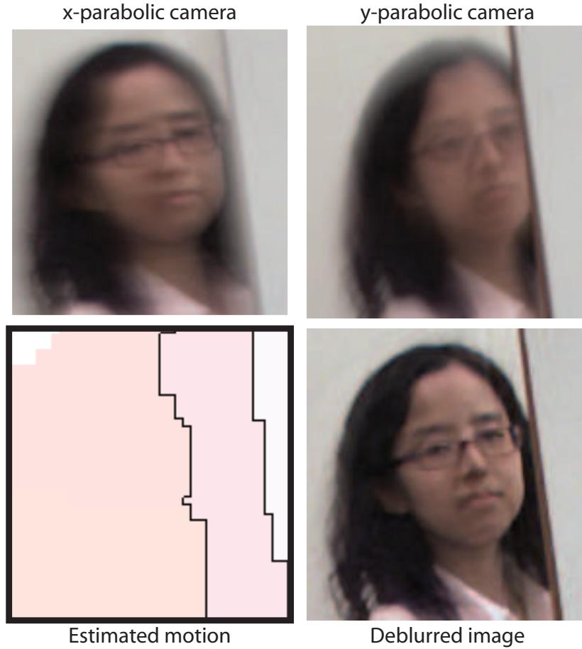
Figure 5.15: Our image reconstruction algorithm handles occlusion boundaries in a manner similar to motion boundaries. In the occluded region, an image deblurred using only one of the two input images is used.
