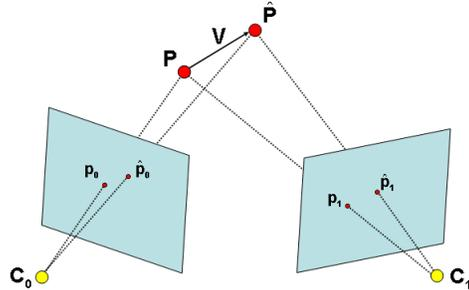
Figure 1. The point  $\mathbf{P}$  is projected to pixels  $\mathbf{p}_0$  and  $\mathbf{p}_1$  on cameras  $C_0$  and  $C_1$ , respectively. The new 3D location at  $t + 1$  is given by  $\hat{\mathbf{P}} = \mathbf{P} + \mathbf{V}$  and it is projected to  $\hat{\mathbf{p}}_0$  and  $\hat{\mathbf{p}}_1$ .
