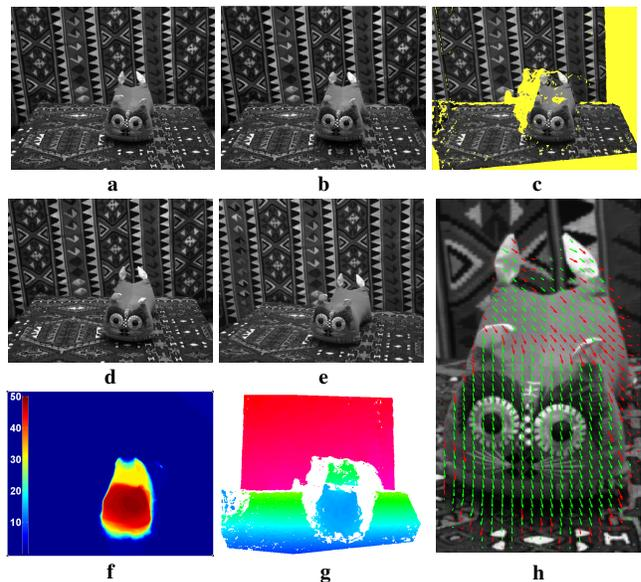
Figure 5. **Cat dataset:** (a,d), the reference view at time  $t$  and  $t + 1$ , respectively; (e), the right view at time  $t$ ; (b,c), warped images from  $d \rightarrow a$  and  $e \rightarrow a$ , respectively; The yellow regions are the computed occlusions; (f), the magnitude of the resulting scene flow (mm); (g), the depth map masked with the computed occlusion maps; and (h), the projection of the computed scene flow. Occluded pixels are colored in red.
