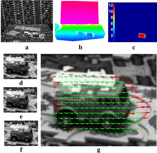
Figure 4. **Cars dataset:** (a), the reference view at time  $t$ ; (b), the depth map masked with the computed occlusion maps; (c), the magnitude of the computed scene flow (mm); (d), zoom in at time  $t$ ; (e), the corresponding warped image; and (f), zoom in at time  $t + 1$ ; (g), the projection of the computed scene flow; Occluded pixels are colored in red.
