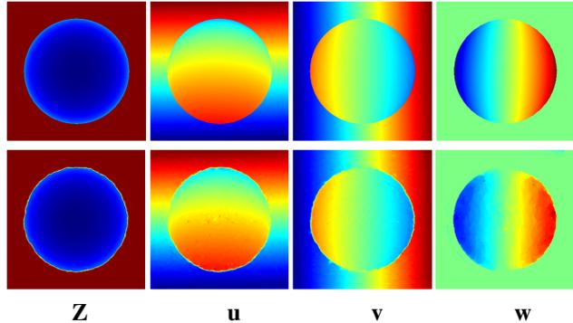
Figure 3. The top figure represents, from left to right, the ground truth for the depth  $Z$  and the 3D motion  $u$ ,  $v$  and  $w$ . The bottom figure shows these results computed by our method.
