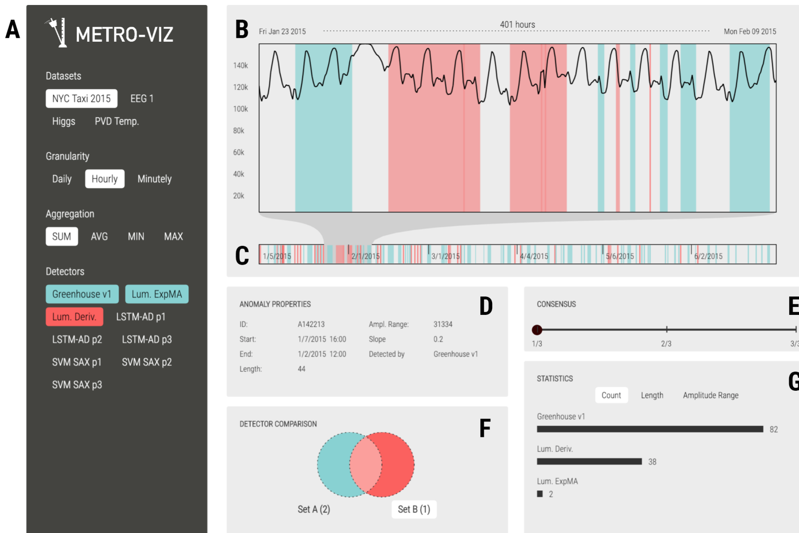
Figure 4: A screenshot of Metro-Viz’s user interface: A) Main menu, B) Time series viewer, C) Time axis showing the full time range, D) Anomaly properties of a currently selected anomaly, E) The consensus slider that can be used to limit the shown anomalies to those detected by a minimum number of detectors, F) The set operation widget that can be used to define and query anomaly sets, G) Summary statistics for all anomaly detectors selected in the menu.
