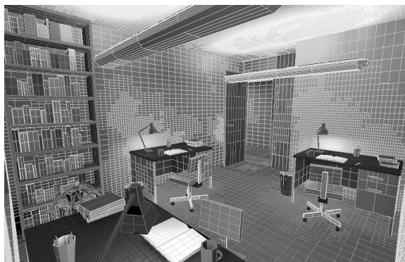
Figure 8: Polygonal mesh generated for the office during radiosity computation.
