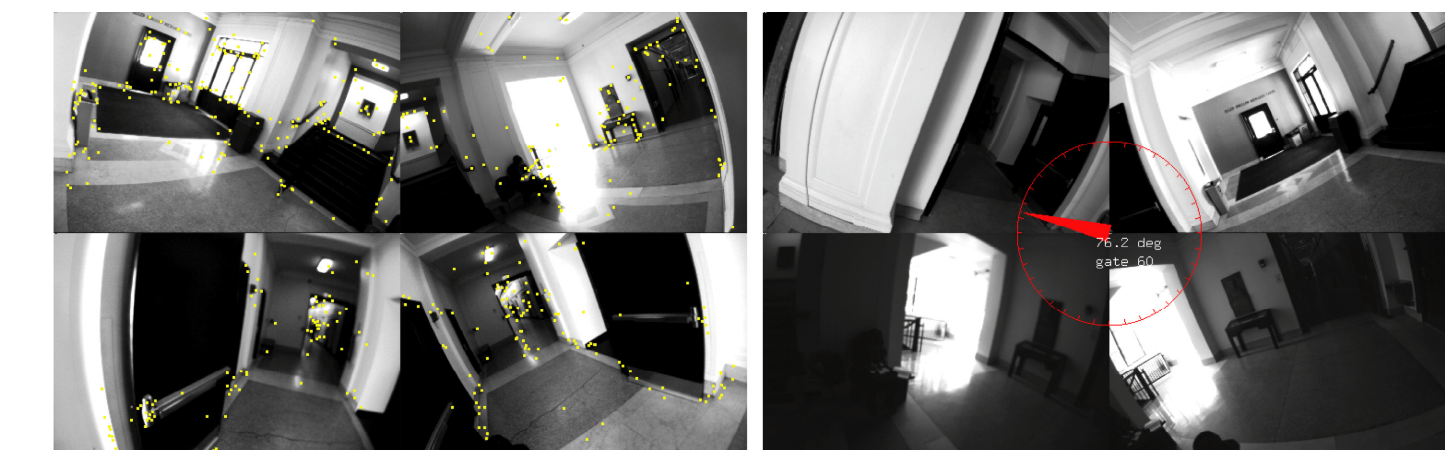
SIFT features (left); body-relative guidance output (right)
