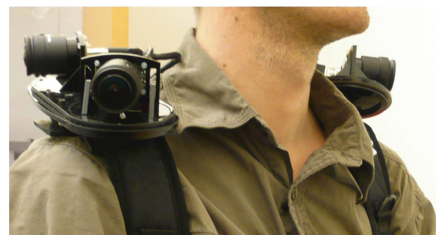
Four Pointgrey Firefly MV; FOV: 360x90 deg
