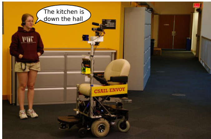
Fig. 1. A user giving a tour to a robotic wheelchair designed to assist residents in a long-term care facility.
