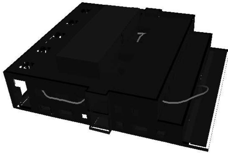
Figure 9.1: The top two floors and roof of the geometric model. The test path (grey) snakes in and out of the building.
