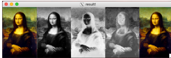
Figure 1: A homomorphic transformation of Mona Lisa from RGB to YCbCr preserves visual similarity. The Y, Cb, and Cr channels are displayed in the middle
