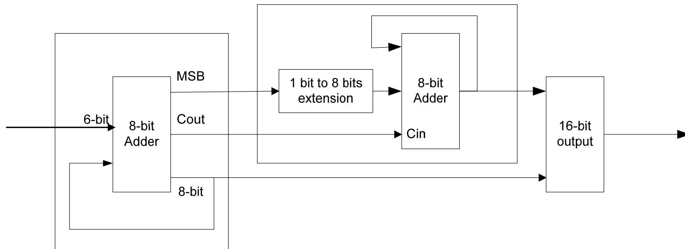
2-Stage Pipelined Accumulator
