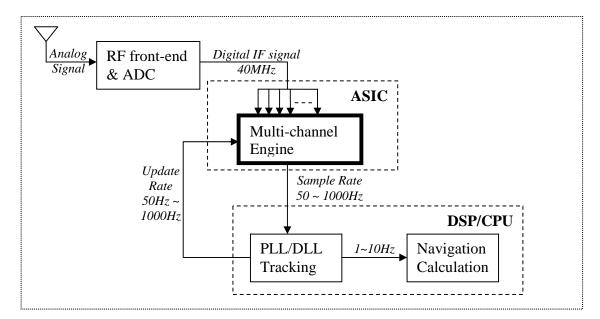
As illustrated in the diagram, the multi-channel engine works on the digital IF signal with a sampling rate of 40MHz as an example. The rate of Pseudo-random (PN) codes embedded in satellite signals is around 1MHz. Thus the over-sampling rate is 40. The multi-channel engine is supposed to handle signals from at least 12 satellites. In our project, we consider one satellite only.
