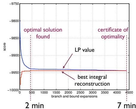
Figure 3: The evolution of the LP value (upper bound) and the best decoded value as a function of branch and bound iterations, for the Alarm problem.
