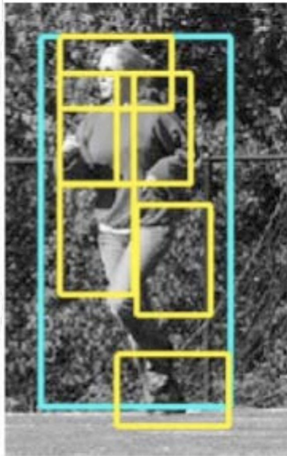
Figure 1. Example detection obtained with the person model. The model is defined by a coarse template, several higher resolution part templates and a spatial model for the location of each part.
