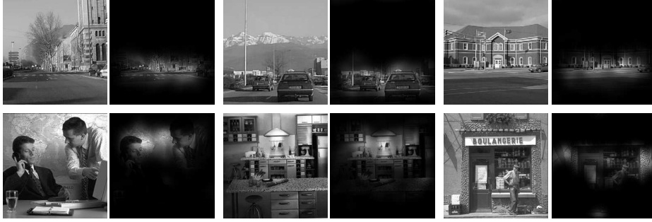
Figure 2: Contextual control of focus of attention when the algorithm is looking for cars (upper row) or heads (bottom row).
