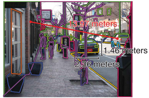
Fig. 13. Snapshot of the 3-D measuring tool. Once we compute the 3-D coordinates for a depicted scene, we can make measurements of scene components. Here, we show the height and the width of the car, which is 13.68 m away from the camera center. We can also compute the distance between any two points in the scene, such as the selected points on the building and the truck.
