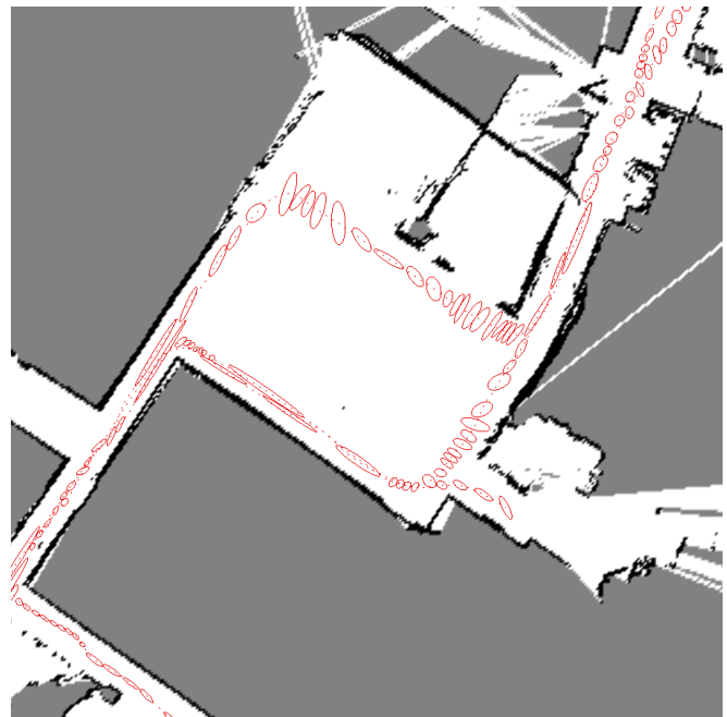
Fig. 7: Predicted covariances for laser scan-matching odometry in a hallway. Note that environmental ambiguity creates large uncertainty along the axis of the hallway
