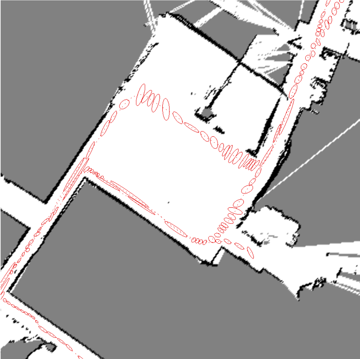
Figure 5-4: Predicted covariances for laser scan-matching odometry in a hallway. Note that environmental ambiguity creates large uncertainty along the axis of the hallway
