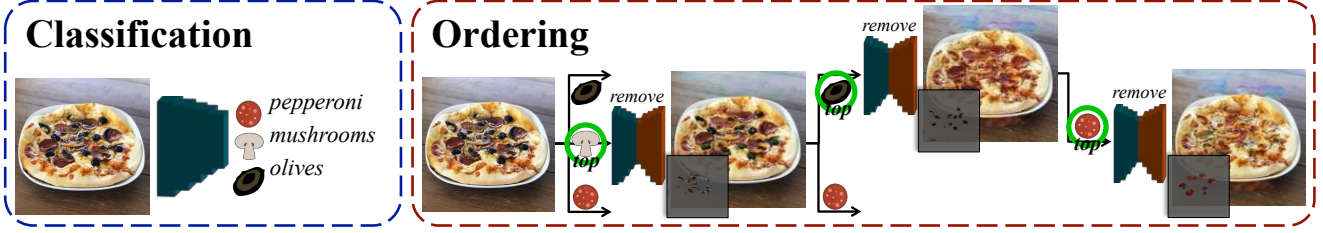
Figure 3. Test time inference. Given a test image, our proposed model detects first the toppings appearing in the pizza (classification). Then, we predict the depth order of the toppings as they appear in the input image from top to bottom (ordering). The green circles in the image highlight the predicted top ingredient to remove. Using this ordering, we apply the corresponding modules sequentially in order to reconstruct backwards the step-by-step procedure for making the input pizza.
